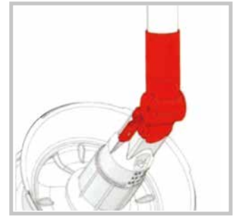
Articulation between feeder and lowering (combination 10+14)
